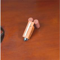
Attach a small amount of the provided removable adhesive to the base the WOLF TERMINATOR. Roll it between your fingers into a noodle as long as the base, as shown in the photo, and press it on.
